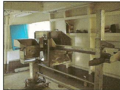
Bait tray loaded with squid (left) and Mini-CircleMatic system (right) installed on longliner.
