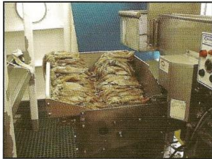
Bait tray loaded with squid (left) and Mini-CircleMatic system (right) installed on longliner.
