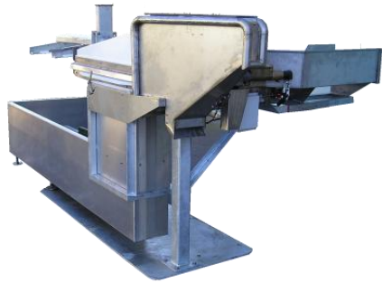
CircleMatic Baiter LCB615 Automatically baits true circle hooks
